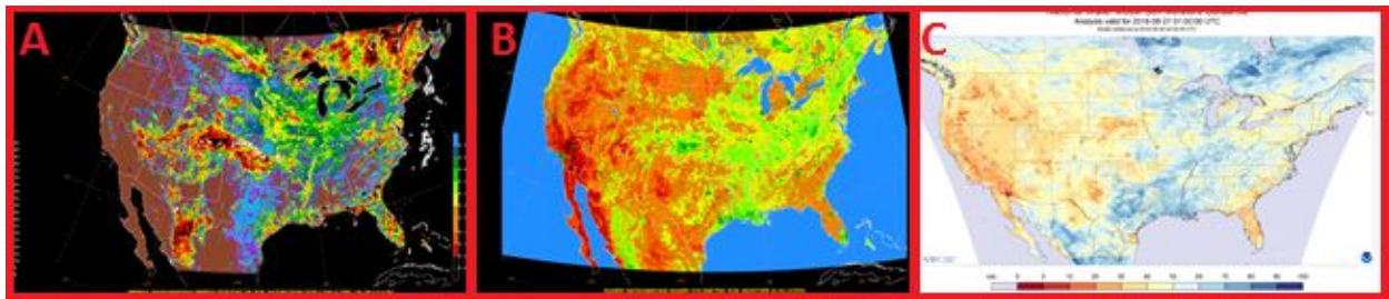
Figure 39. Examples of soil moisture products offered, including (a) Percent Soil Saturation for 0-1 cm from the ESRL HRRRv2, (b) the Volumetric Soil Moisture for 0-10 cm from the NAMRR, and (c) the Soil Moisture for 0-40 cm from the National Water Model.
